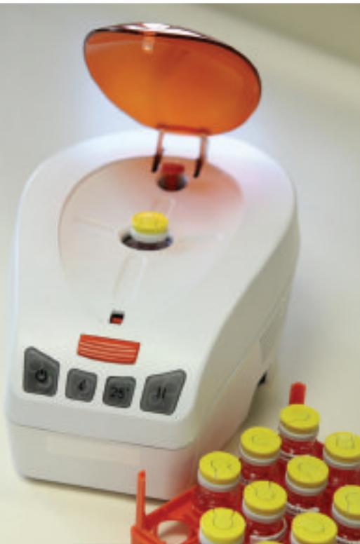
**Figure 2:** A device for rapid and precise thawing of cell vials at the point of care
